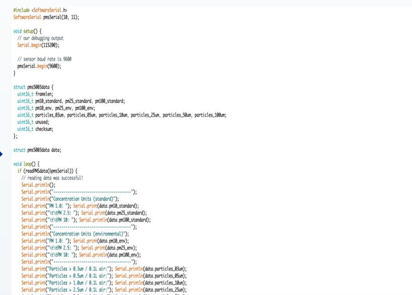
Arduino code to collect Particulate Matter levels and print them on the laptop
