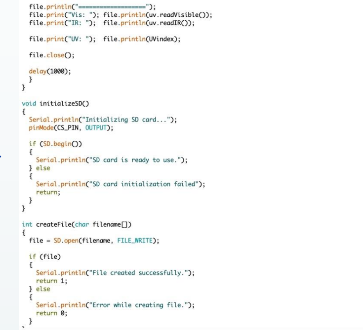
Using the Arduino IDE to code each sensor and their corresponding SD card
