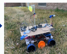
All Arduinos and corresponding sensors mounted onto TerraRover 2
