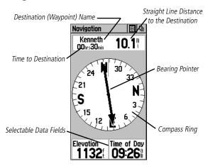
The Navigation Page provides active guidance with a rotating compass ring that shows your course over ground (track) while you're moving and a bearing pointer to indicate the current direction to your destination (bearing) relative to the course over ground.
