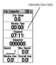
The Trip Computer Page displays up to eight different types of navigation data and are user programmable. Each data field is selectable and can contain one of many data information options. The default settings for these fields are shown in the illustration.
